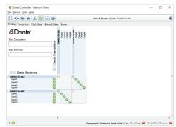
Next, configure audio interface and device name of Dante Virtual Soundcard using Dante Controller. By default, the device name of Dante Virtual Soundcard is user name of your computer.
